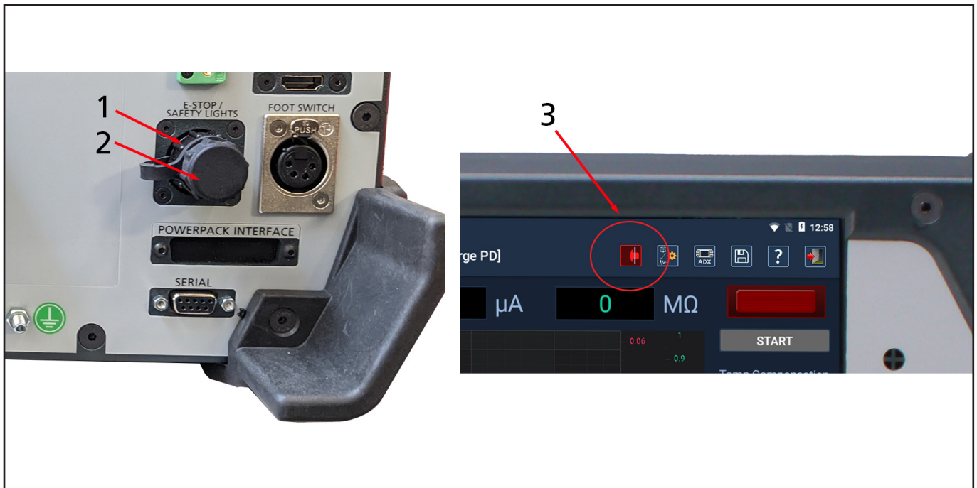
Fig 7: Stop Jumper connectors and cover (left). E-stop indicator in ADX test screen toolbar (right).
