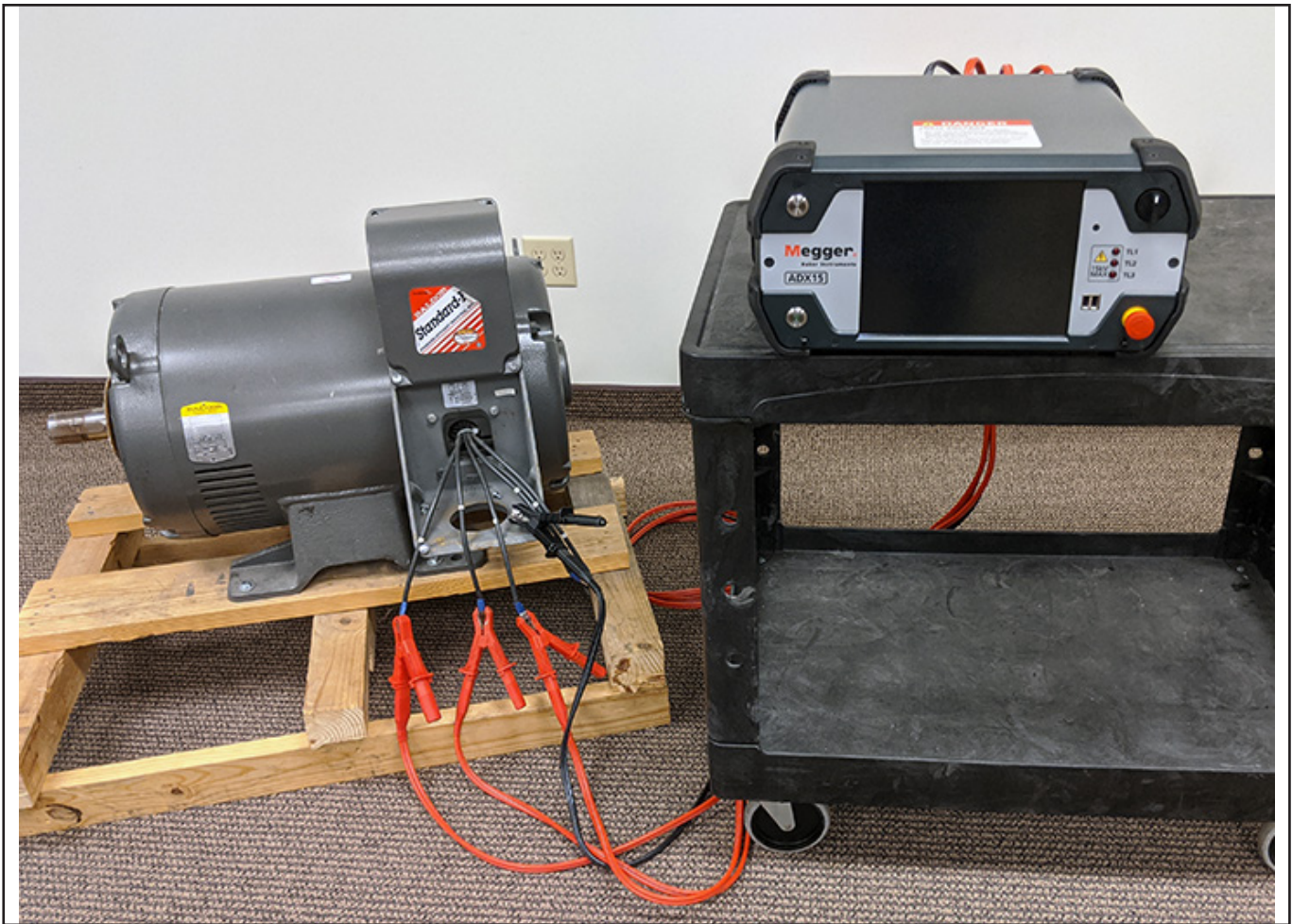
Fig 28: Ensuring ADX test leads and Asset cables are properly separated and located.
