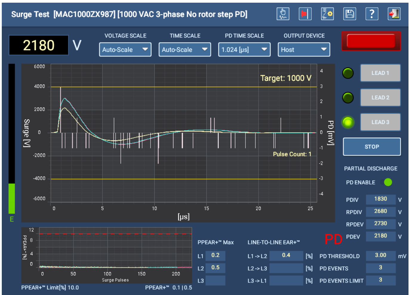
Fig 114: Voltage dropping to ramp down target (1000 V here), capturing extinction values for Lead 3.
