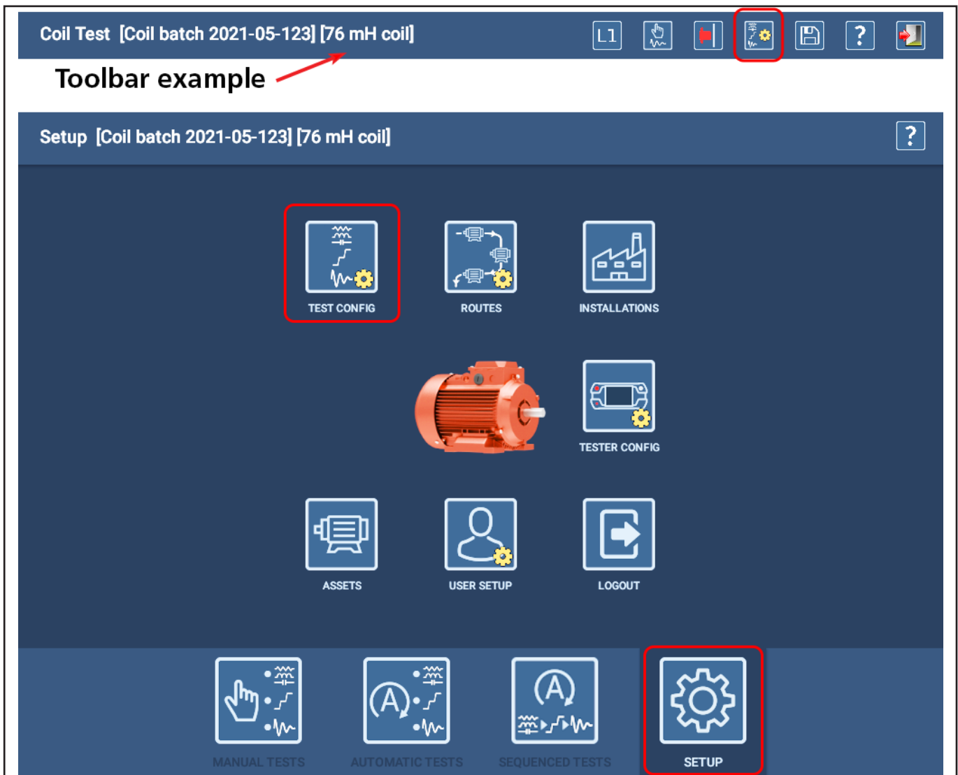
Fig 41: Access Test Configuration Editor from Setup Main or icon at top of many test screens.
