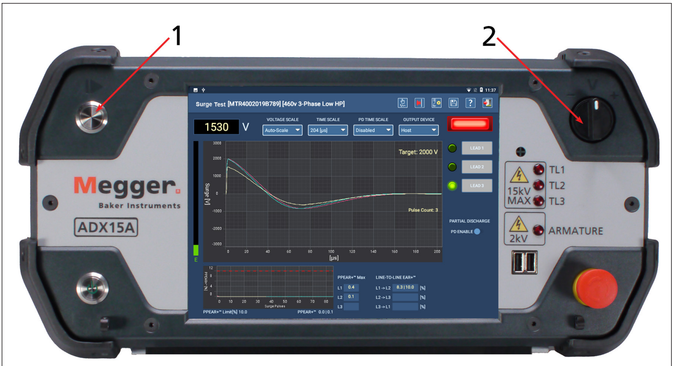
Fig 88: ADX front panel controls for starting Surge test.
