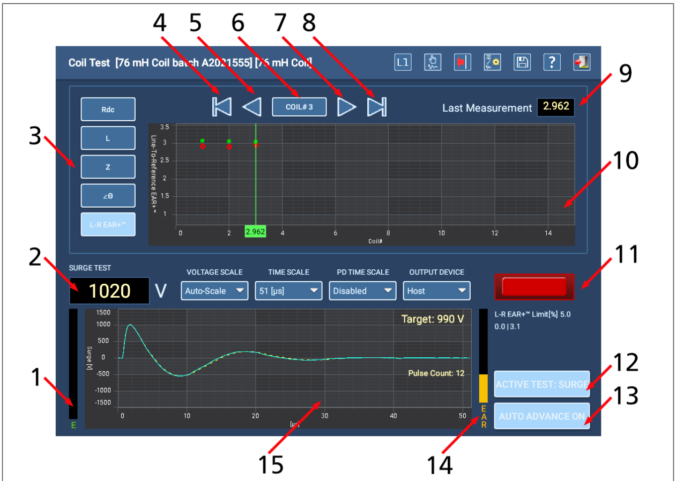
Fig 98: Coil Test screen elements.
