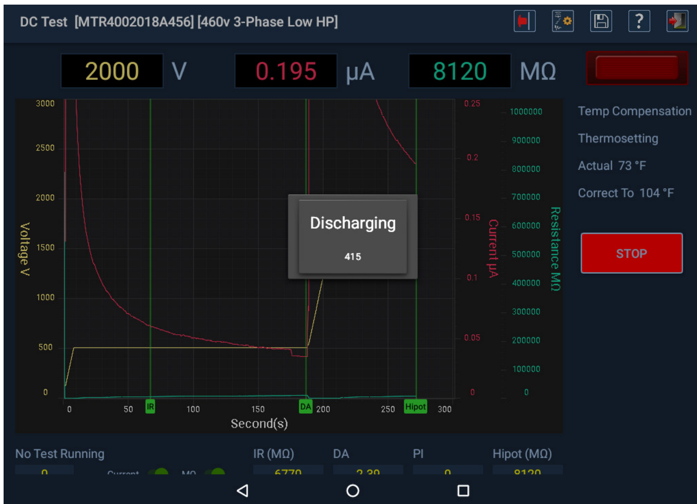
Fig 109: Auto DC Test completed and displaying discharging message box.
