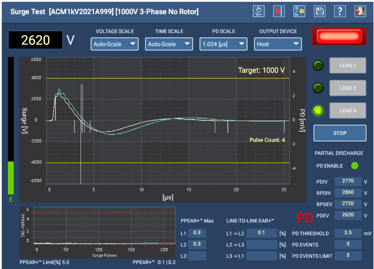
Fig 118: Surge testing with PD in Automatic Mode to confirm settings.
