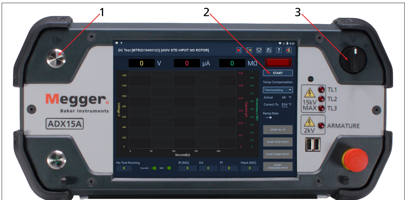
Fig 85: ADX front panel and user interface controls for starting DC test.
