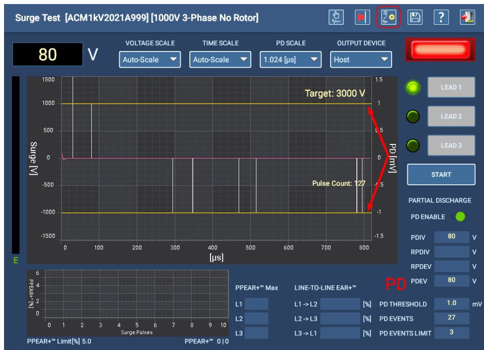
Fig 116: Surge Test screen in Manual mode for setting PD parameters.
