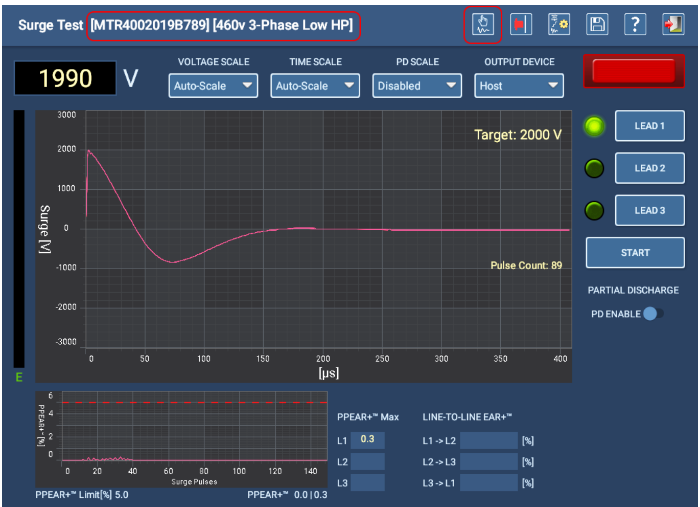
Fig 89: Acquiring reference waveform for Surge Test on LEAD 1.
